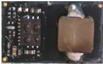
Figure 16. PCB of the power module with selected metal powder composite inductor.
